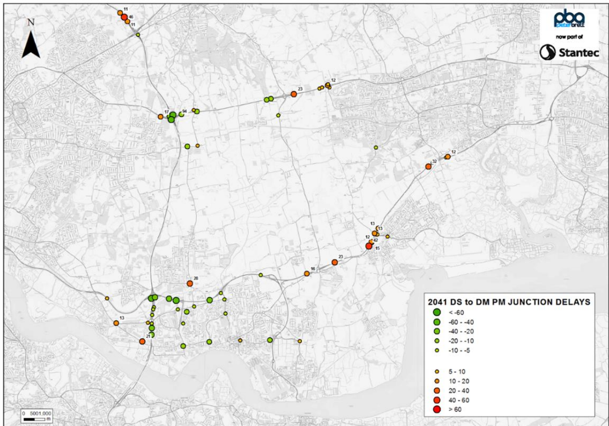
Figure 6.2: Differences in Delays in PM Peak Hour with LTC (Statutory Consultation Fixed Matrix Cordon Model)
